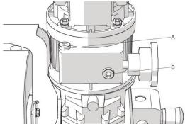
Fig.6.3.1 There are several grease nipples on the UZ30 machine (Fig. 6.3.2) that must be kept clean and filled with lubricant at least once a week. Recommended grease Shell Alvania RL 2 The recommended lubricant is Shell Alvania RL 2.
