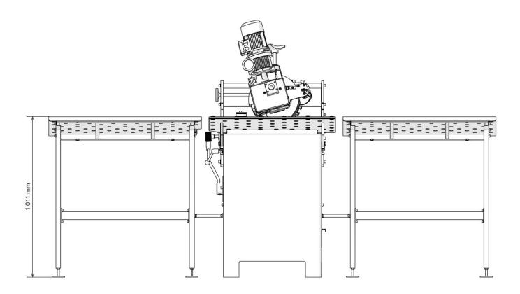
Important: Caution when installing the adjustable support rulers (position B Fig. 7.1.1.). Shorter ruler must be mounted on the left table provided with a recess for easier access to regulate the angle and the sliver, as indicated in Fig. 7.1.1.
